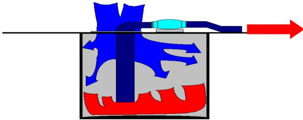
**Ventilation of a single top opening vessel**
