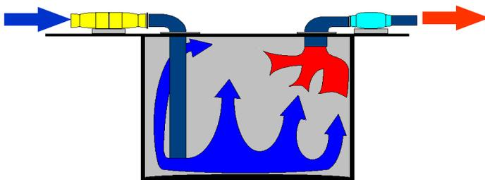
**Removing lighter than air contaminants, dual opening vessel.**
