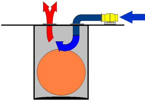
**Short circuiting** the air flow by not introducing the fresh air flow deeply enough within the space. Use extension ducting to avoid this.
