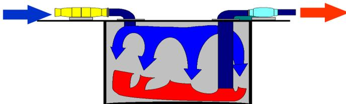
**Removing heavier than air contaminants, dual opening vessel.**
