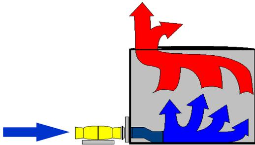
Ventilation of a **deep confined space** should introduce air at the lowest point possible with the contaminated air exhausted to the top. This can be achieved by an access through a low point or by directing air into the low part of the tank via ducting.
