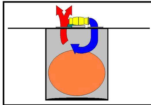
**Recirculation** of contaminated exhaust back into the space by having the blower too close to the exhaust position.
