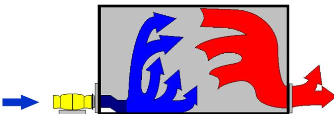
Ventilation of a **Long Confined Space** can be achieved by blowing fresh air in at one end and exhausting the contaminated air at the other end. In the case of the example here, unless the airflow is *directed up* into the 'dead zone', you will get a situation where the ventilation is short-circuited.
