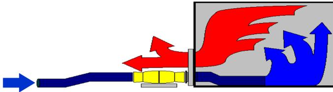
If the entry and exit spaces are close together or the same access point, by blowing fresh air *deep* within the space using ducting and allowing exhaust air to be pushed out of the exit. In this case the introduced air must be protected from the exhausted air by attaching ducting.
