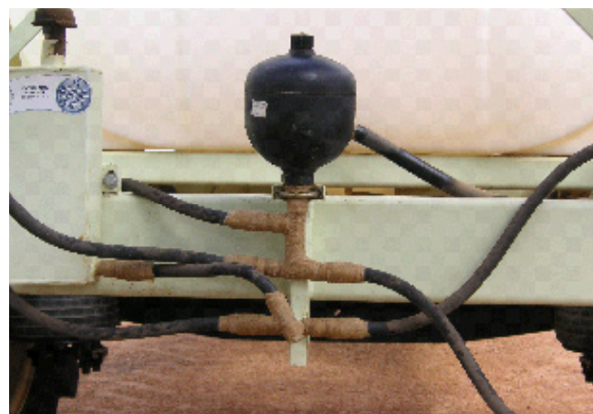
Susceptible materials on a boom sprayer protected from corrosion using Denso Tape.
