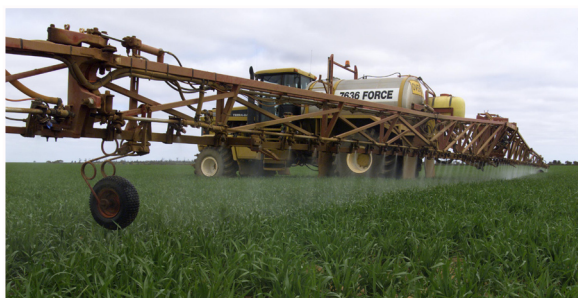
Boomsprayer applications of Flexi-N provide even coverage right to the edge of the paddock compared to topdressed urea.
